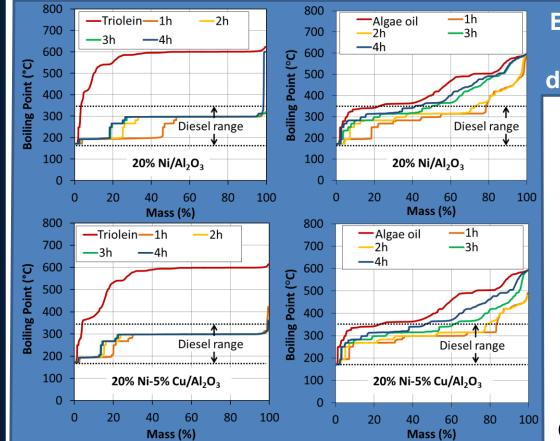
Boiling point distribution plots of two feeds and their continuous deoxygenation products at 260 °C
