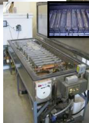
Freezing and thawing testing
