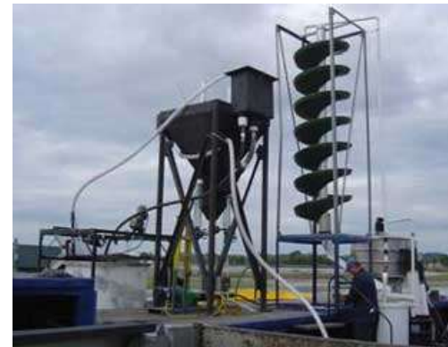
Density separation – Spiral Method
