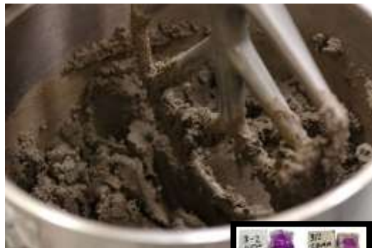
Production of mortar in a Hobart mixer
